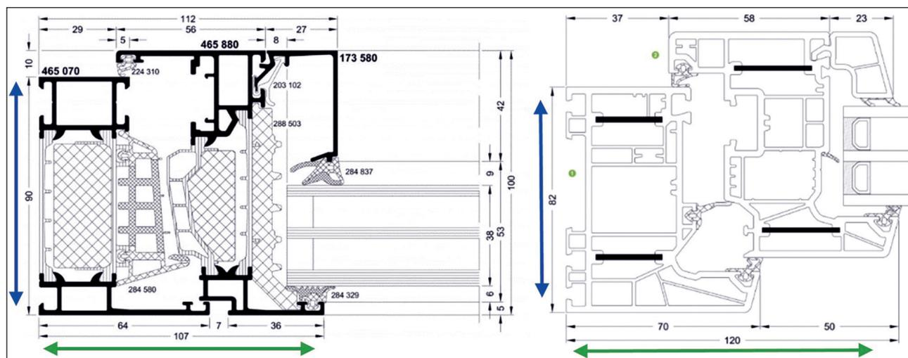
Figure 1. On the left side cross-section of aluminium window and on the right side cross-section of PVC-U window (Schuco, 2020)
