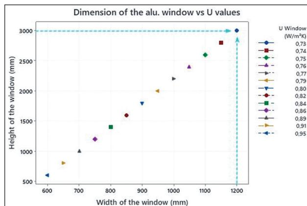
Diagram 3. Aluminium window size results of testing
