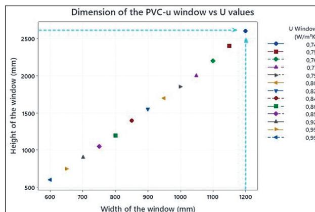
Diagram 4. PVC-U window size results of testing
