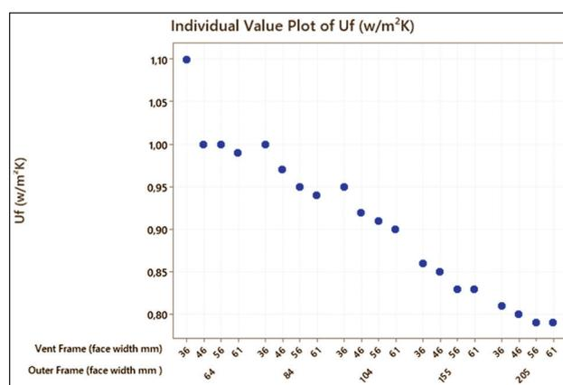
Diagram 1. Profile combination for aluminium frames results of testing
