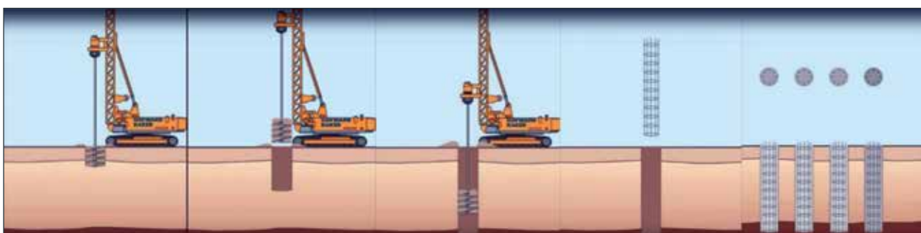
Figure 3. The technology of reinforced concrete piles used in excavation and protection of construction pits [4]
