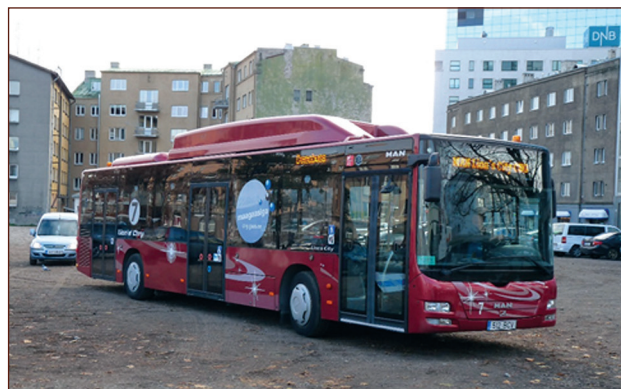
Picture 1. MAN vehicle for public transport with earth gas drive
