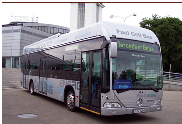
Picture 2. Mercedes-Benz O530 Citaro vehicle for public transport driven by hydrogen combustible cells (Brno, Czech Republic)
