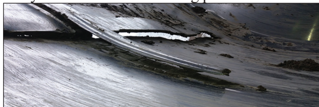
Figure 11. Characteristic damage to excavator bucket segments
