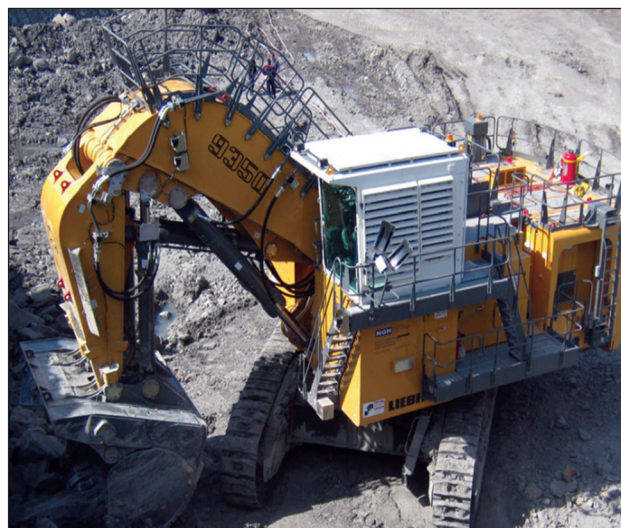
Figure 4. Hidraulic excavator Liebherr R9350
