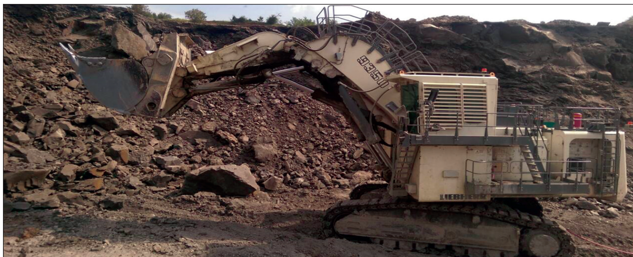
Figure 10. Bucket in fully extended horizontal position
