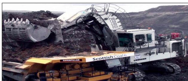
Figure 3. Hydraulic excavator in working position
