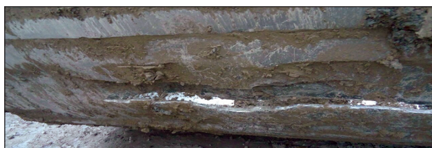
Figure 12. Characteristic damage to the excavator bucket segment
