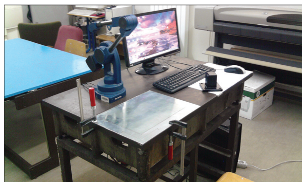
Figure 2. Positioning the flat panel on the measuring table as a preparation for digitalization by tactile scan
