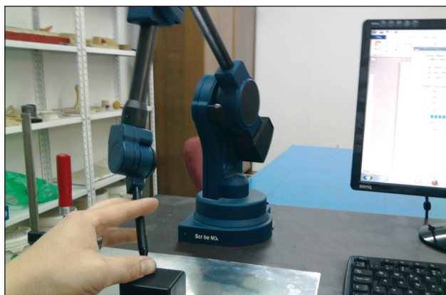
Figure 3. Contact scanner - device for digitalization with the appropriate calibration gauge mounted on the measuring table
